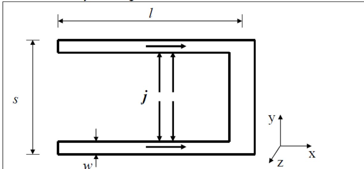
**figure 1:** cut-out of the top view on the front-grid. The grid consists of a thick busbar, in which the losses can be neglected, and of several (of which only two are depicted here) equidistant fingers with length  $l$  and width  $w$ . The distance between two fingers is  $s$ .
